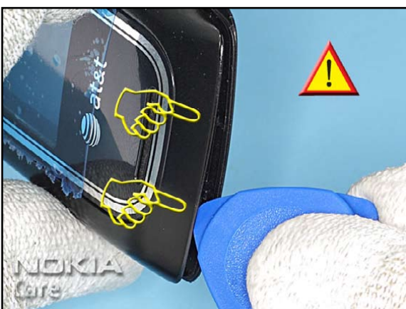
11. Now, release the two top clips of the A-COVER beginning on the rounded side of the cover.
