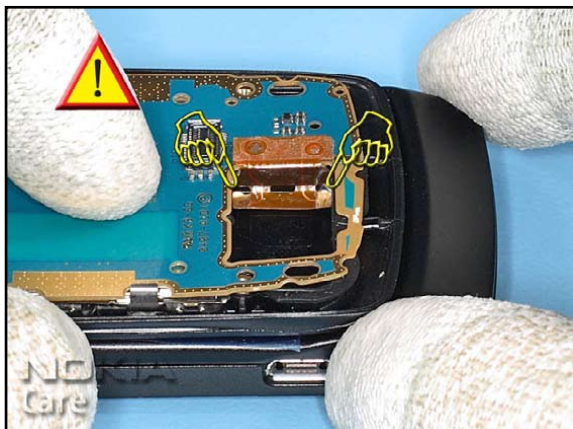
13. Ensure that the flexible contacts for the IHF SPEAKER are also positioned correctly.
