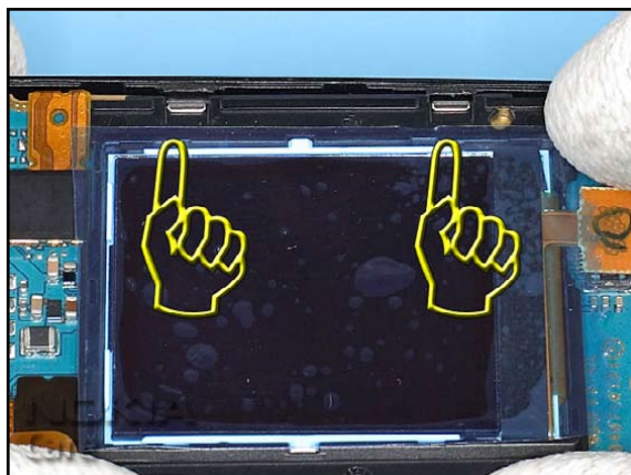
16. Fit the shown side of the LCD into the B-COVER ASSY and close the LCD connector.
