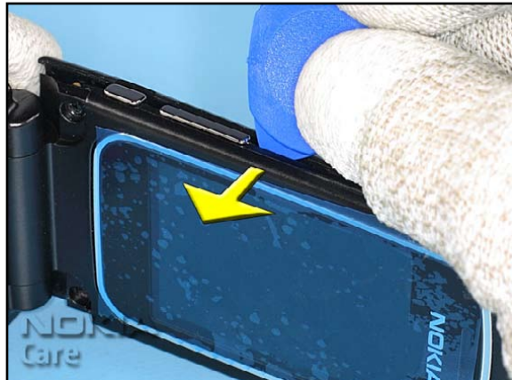
8. Unlock the clip in the middle...
