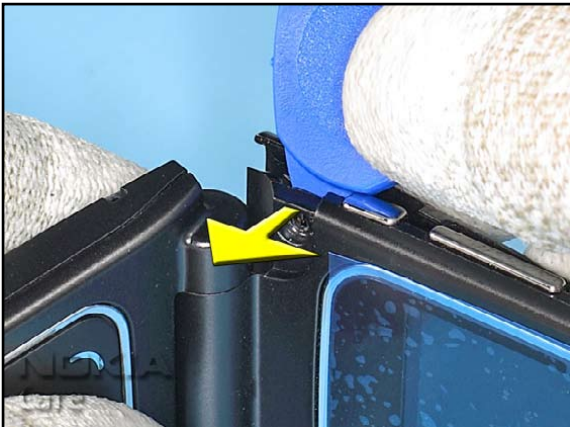
7. Unlock the clips of the A-COVER starting on the HINGE side.
