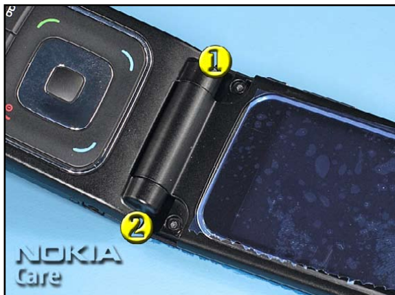
24. Always use new screws when assembling the unit. Tighten the screws to the torque of 14Ncm in the order shown.
